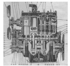
FIG. 2 -- SIDE SECTIONAL VIEW OF ENGINE
